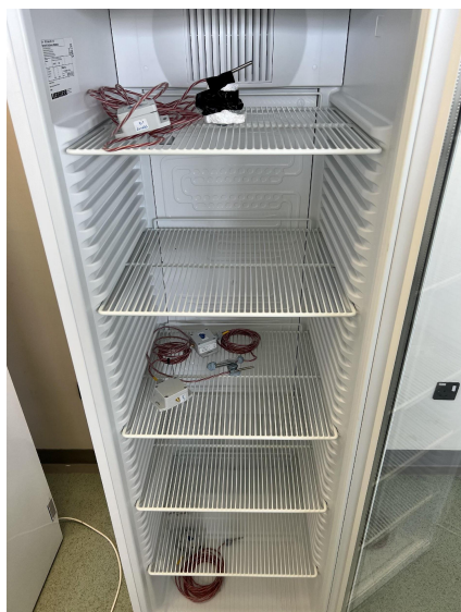
Figure 2. Probe positioning inside the LKv3913.
