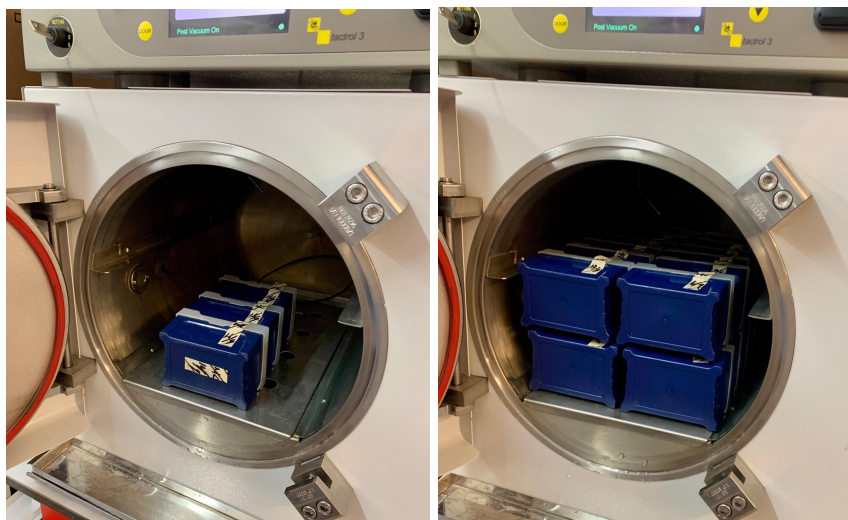
Figure 2. 'Minimal' loading (left) and 'maximum' loading (right) of the Compact 40.
